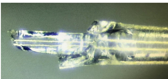
(e) 48 h 后裂纹扩展、断裂
